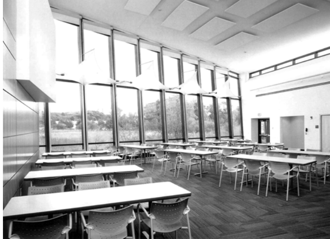
Figure 5-2 Example of north-facing assembly space that optimizes daylight harvesting while minimizing solar gain.
